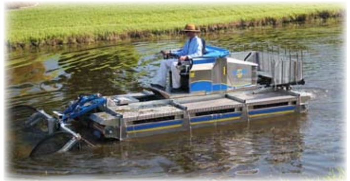
Above: The Truxor cuts and harvests invasive vegetation in our canals. Below: FloridaAquatic President John Farrell at work harvesting weeds. Photos by Wayne Mengel (top), Sue Killion (below).
